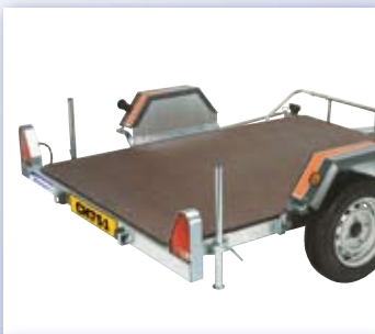
Phenolic plywood decking
